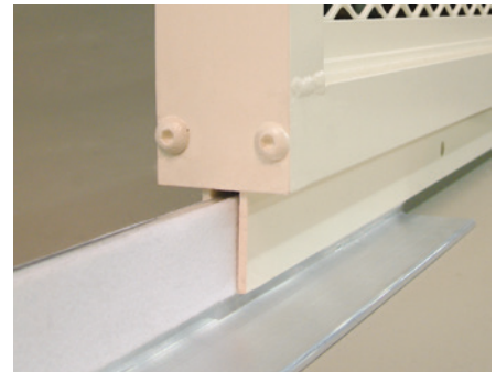
Smooth Guidance - A floor-anchored aluminum guide angle with conservation-safe felt eliminates metal to metal contact reducing vibration.
