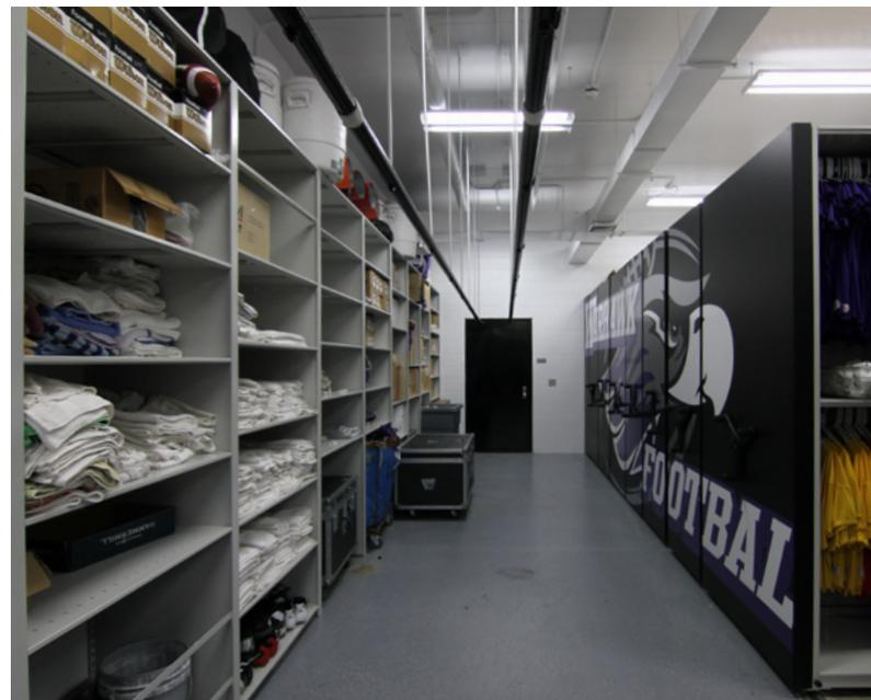
Storage compartments within the stationary 4-post shelving units were designed for balls, towels, and other more frequently accessed gear that did not need to be secured.
